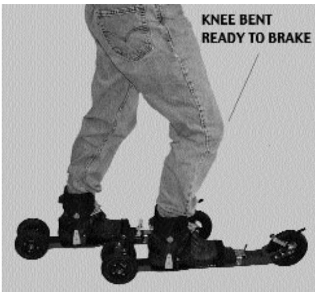
**Preparing to Brake:** Position for getting ready to brake. The braking foot should be about 18 inches, 0.4 meters, ahead of the other foot with the knee pushed slightly forward. This is called a Telemark position which is a very stable body position for braking.
