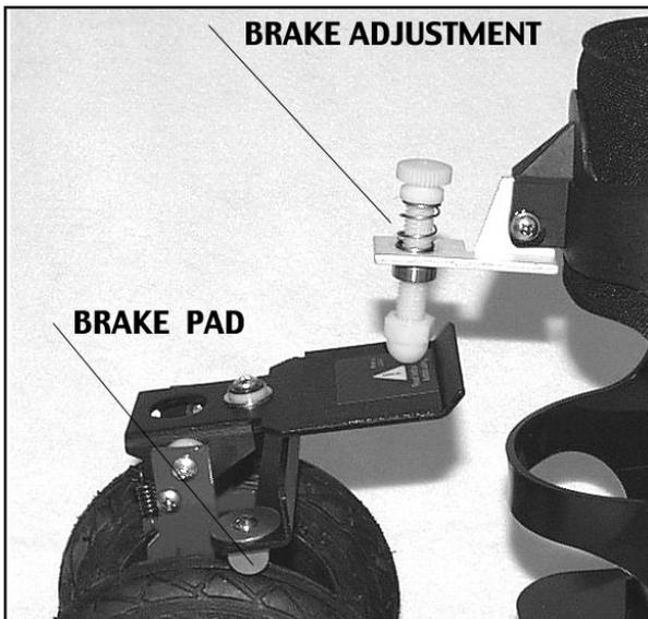
**Brakes:** Brake adjustment can be made with the plastic Thumb Screw, see photo. Adjust the brake so the brake pad is not dragging against the wheel when skiing normally. To brake place the brake foot about 12" to 18", in front of the other foot and push your knee back as shown in the pictures below. This motion causes the cuff to pivot and the brake adjustment arm engages the brake platform and the skis come to a smooth stop.
