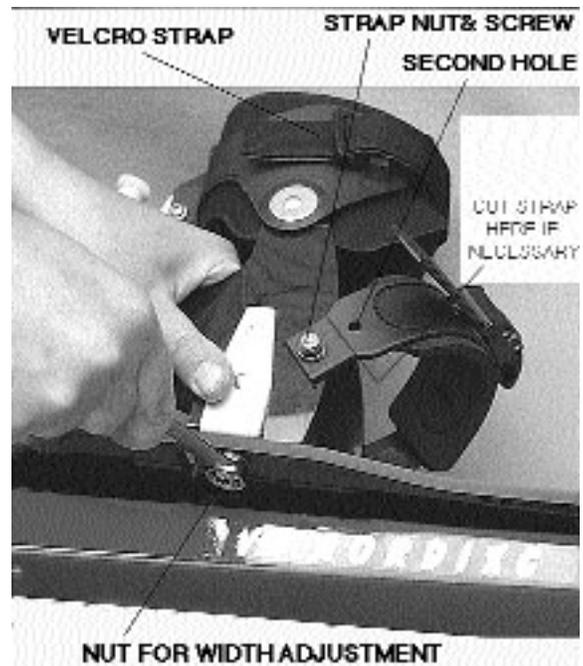
**Width Adjustment:** For good control when skiing, the width of the foot support should be adjusted so the bottom of the foot support is snug against the shoe. To adjust loosen the nut using a 11mm or 7 / 16" wrench, reposition and tighten. **Make sure you adjust from both sides so the foot support is centrally located on the platform.**
