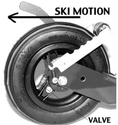
**TRACKING:** The chassis is designed so that you can slightly alter the tracking of the ski. One hole on the front wheel fork, the side where the nut is mounted, is slightly obround. If the ski pulls to one side, loosen the nut about 2 turns and while pushing the wheel against the table top in the opposite direction of where the ski wants to "pull" retighten the nut. The serrated washer under the nut on the front fork will keep the wheel from shifting back to the center of the hole.
