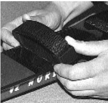
To move the toe stabilizer lift at rear as shown in the photo and slide forward or backward. The unit is spring loaded so the rear can be lifted. When the toe stabilizer is in the proper position make sure the pegs on the stabilizer are in the holes of the platform.
