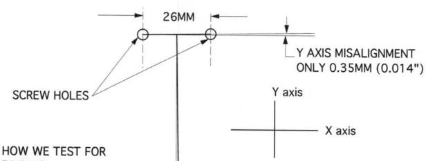
HOW WE TEST FOR BINDING MISALIGNMENT
