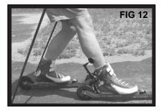
Using the Brake: FIG 12: Practice braking on flat surfaces and very gentle slopes. To use the brake, move the braking leg ahead of the other like a ski jumper coming in for a landing. Press your calf against the yoke until the brake pad contacts the wheel. After you have practiced on gentle slopes try steeper terrain and see if the brake position needs adjustment.
