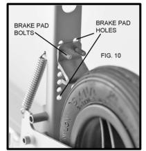
Adjusting the brake to suit your anatomy: In the vertical position mount the brake so the yoke is above the boot. Most skiers prefer the yoke to be
