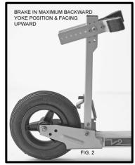
The yoke has seven horizontal adjustments (**FIG 2 and FIG 4**) and can be mounted straight by mounting the screw in the lower position of the two intersecting holes. (**FIG 3**). By mounting the screw in the upper position of the intersecting holes the yoke is angled upward as shown in **Figures 2 and 4**.
