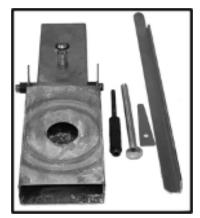
The Tire station shown should be mounted on a bench as close to the edge as possible. The Tire Station must be securely fastened to the work bench via the 4 screw holes. For a less permanent fixture, you can mount the Tire Station to a plank of wood, then clamp the plank to the edge of a strong table or sawhorse when in use.
